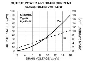
RoHS Compliance, 400-470MHz 30W 12.5V, 3 Stage Amp. For MOBILE RADIO
