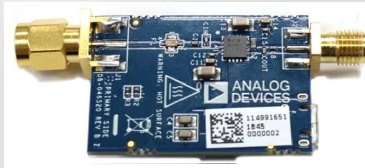
USB Powered 2.4 GHz RF Power Amplifier
