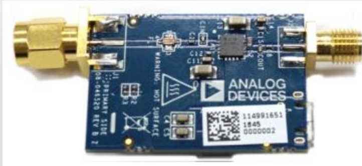
USB Powered 2.4 GHz RF Power Amplifier , Analog Device CN 0417 - Gain: 20dB
